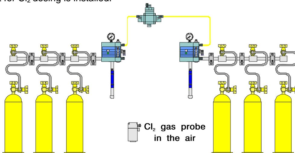
Typical use of chlorine gas in the air probe
